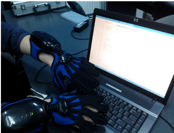
Fig.1.50 HandTutor attached to computer [73]
