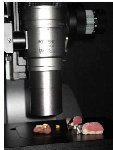
Fig.2.33 Keyence digital microscope (500x) [59]
