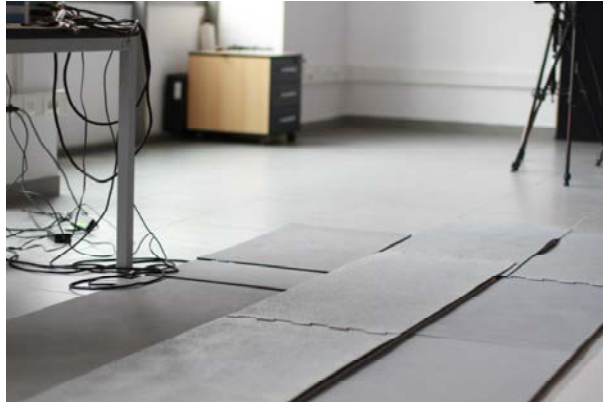
Fig.1.36 Plantar pressure platform covered with plastic rugs [71]
