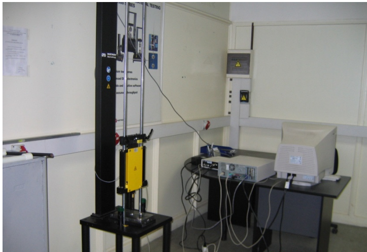
Fig.2.75 Impact testing equipment with acquiring data system [54]
