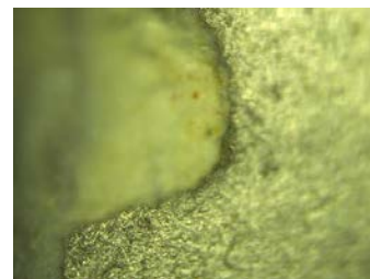
Fig.2.40 Acrylate on metal support tooth sample after 144 hours of immersion in natural juice (left) and instant coffee (right) [59]
