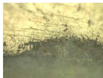
Fig.2.41 Acrylate on metal support tooth sample with abrasions and small cracks before immersion in coca-cola and same sample after 144 hours [59]
