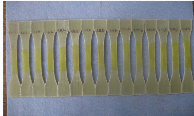
RT300 glass fabric-reinforced Polylite 440-M888 polyester resin specimens cut on weft direction
