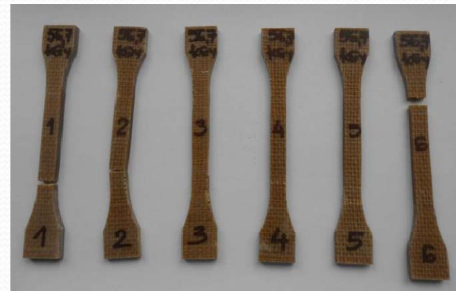
Hemp fabric based specimens irradiated with 56,7 kGy dosis
