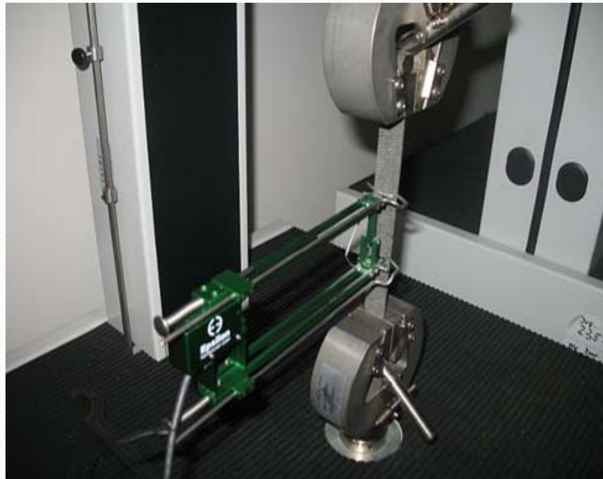
Tensile test detail on an epoxy impregnate 2/2 twill weave carbon fabric
