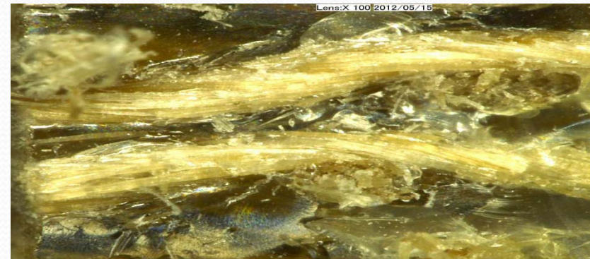
Cross-section through a hemp fabric based specimen irradiated with 56.7 kGy dosis (100X magnitude)
