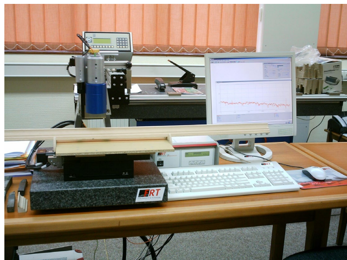
Fig. 60. Equipment for measuring the roughness of surfaces with an optical beam
