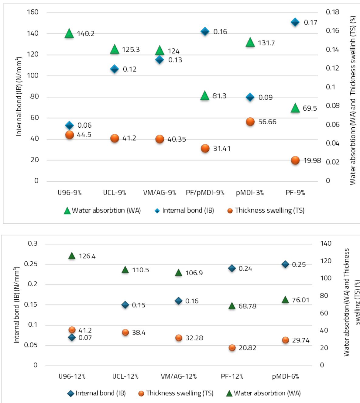
Fig. 18. Effect of adhesive type and content on thickness swelling (TS), water absorption (WA) and internal bond strength (IB) of modulus of elasticity (MOE) panels (according to Zeleniuc et al. 2019)
