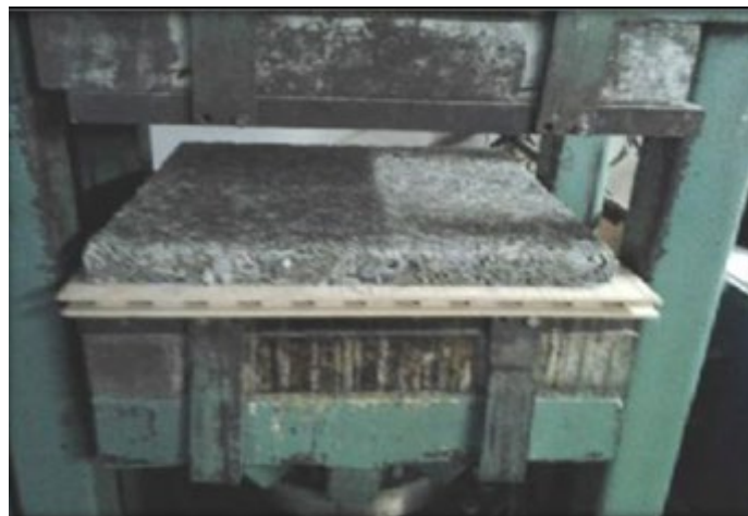
Fig. 33. Pressing of composites (Brenci et al. 2014)
