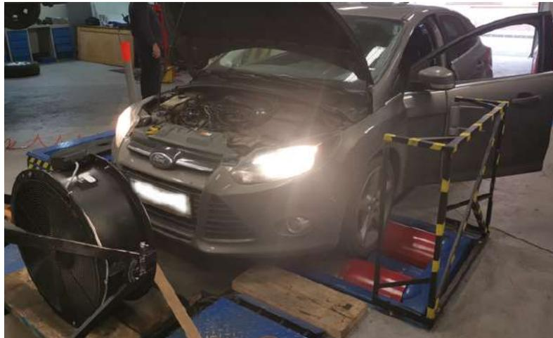
Fig.1 The dynamometric MAHA LPS 3000 test bench
