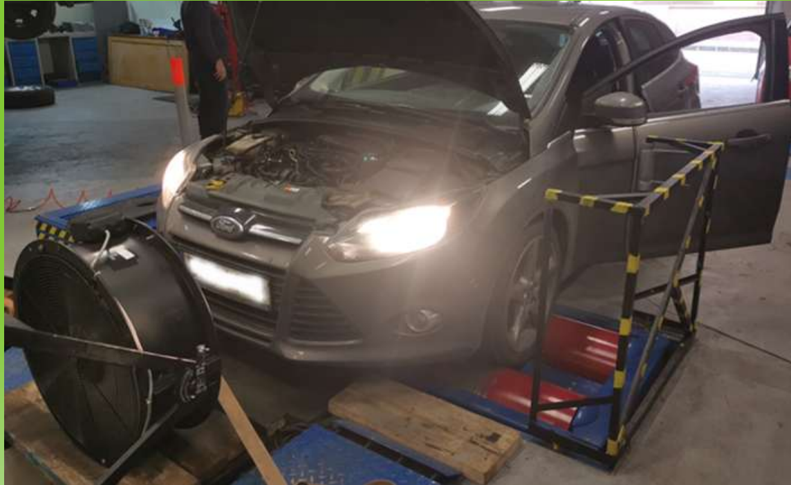
The test car on the dynamometric MAHA LPS 3000 test bench
