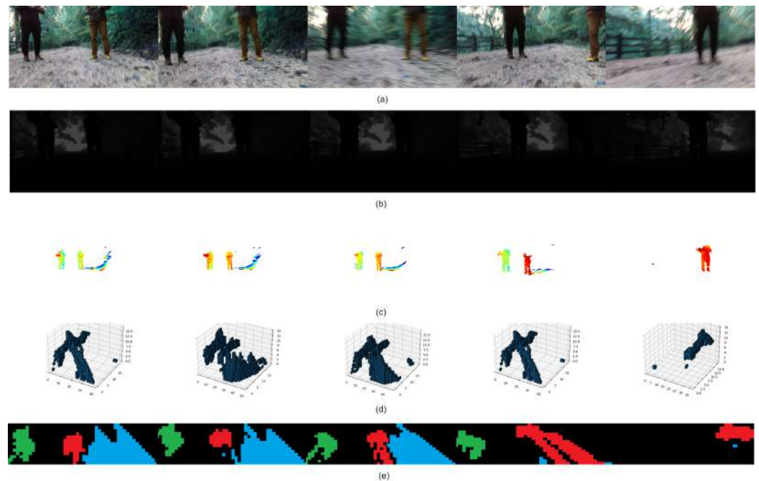
Figure 5. Experimental data processing chain. The experimental data used by the algorithm. From top to bottom: (a)—RGB data, (b)—depth image, (c)—3D representation, (d)—3D voxel grid, and (e)—2D voxel grid.
