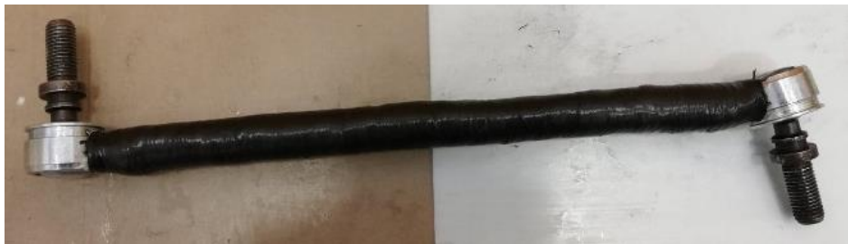
Figure 38 The CPET weave is covered with heat shrink tape
