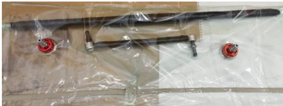
Figure 39 Hybrid connecting rod in the vacuum bag prepared for the thermal consolidation process
