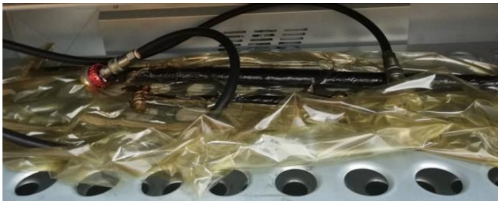
Figure 40 Hybrid connecting rod in the oven, at the end of the consolidation process
