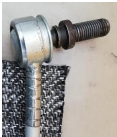
(c) C/LPET weave wrapped around the steel end and aluminum tube
