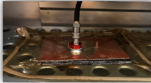
Consolidation under vacuum at 200°C
