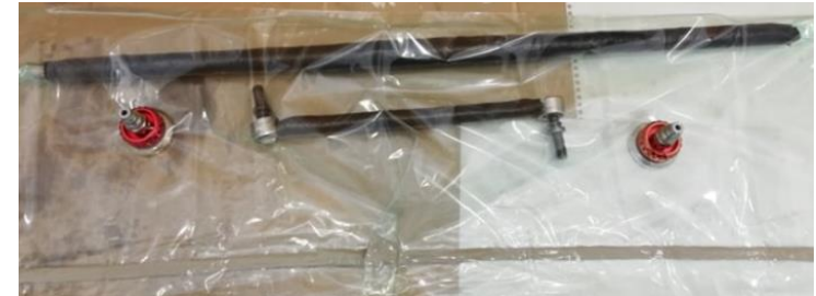
Hybrid connecting rod in the vacuum bag prepared for the thermal consolidation process
