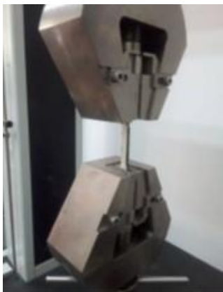
Figure 8 Specimen during tensile testing Fig.9 Tensile testing in graphic (mechanical characteristics)
