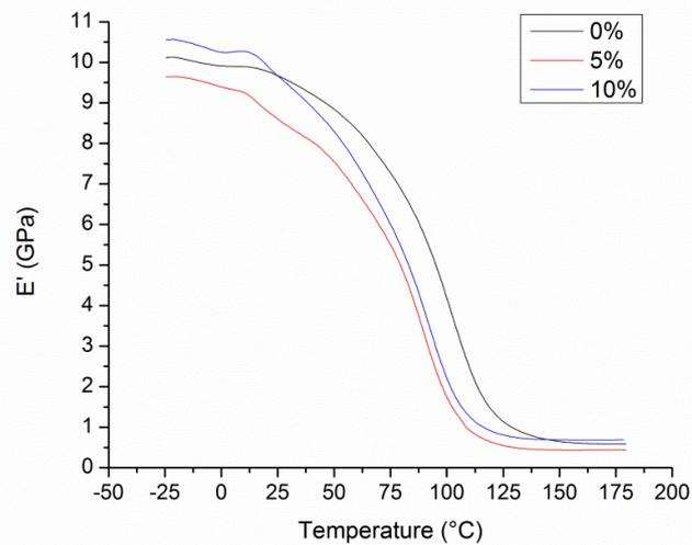
Fig. 16 Particle content effects on the storage modulus at different temperatures
