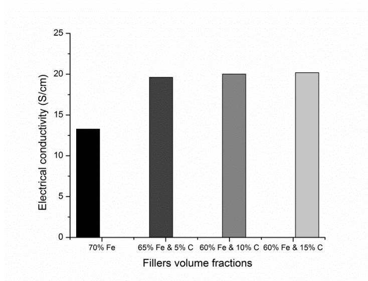
Fig. 56 *Effective predicted electrical conductivity values for a 0.2 percolation threshold*
