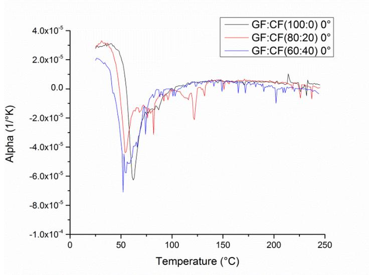
Fig. 45 Instantaneous effective CTE variations with temperature
