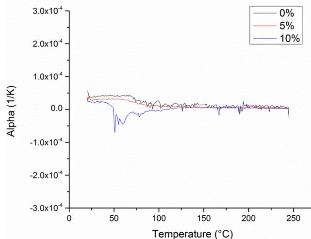
Fig. 29 Overall CTE temperature variations after water exposure along 1 week
