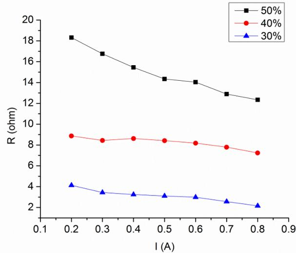
Fig. 52  $R(I)$  variation for different volume fraction of iron particles
