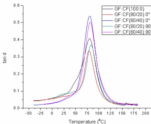
Fig. 25 Damping factor variation with temperature and UD fiber orientation in fiber-fiber hybrid composite architectures
