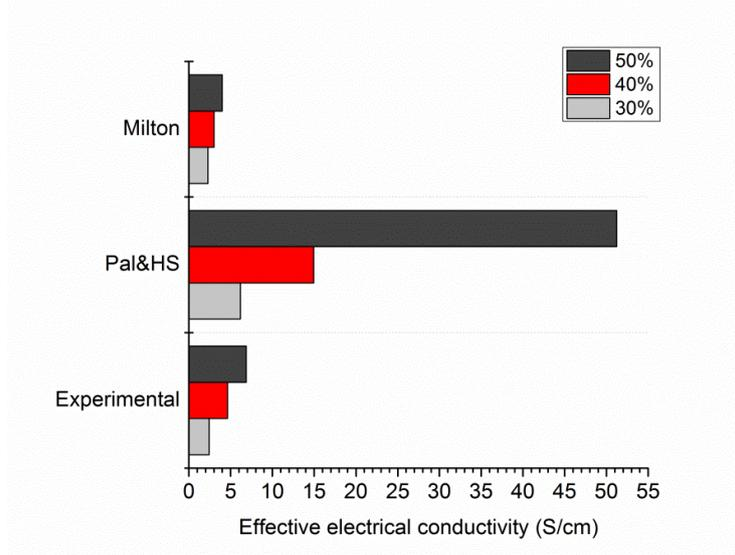
Fig. 53 *Comparative theoretical-experimental data on effective electrical conductivity for different relative content of iron particles*
