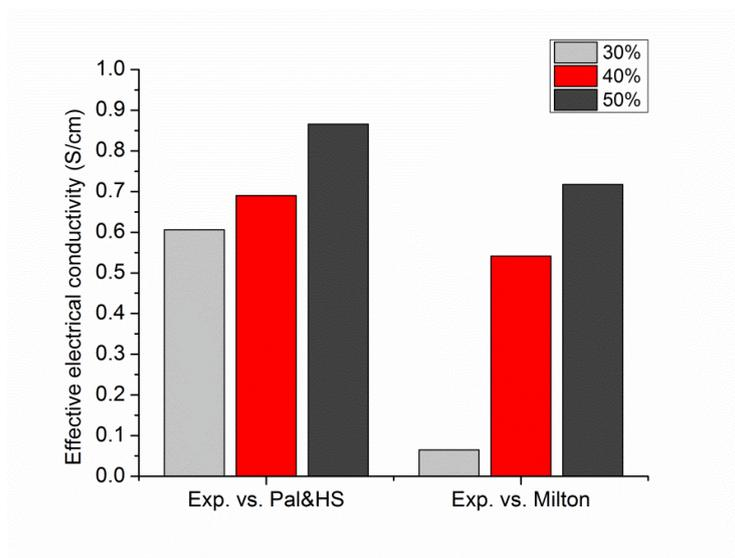
Fig. 54 *Absolute values of relative percent error from experimental and predicted values on effective electrical conductivities of hybrid composites*
