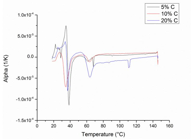
Fig. 49 Instantaneous CTE variations with temperature during the heating step
