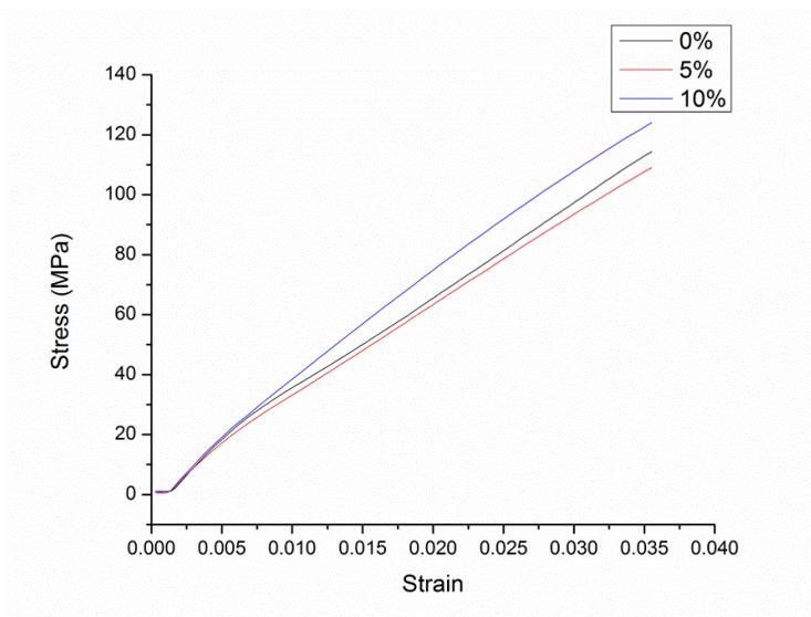
Fig. 5 Stress-strain curves from tensile tests on ceramic fillers hybrid composites
