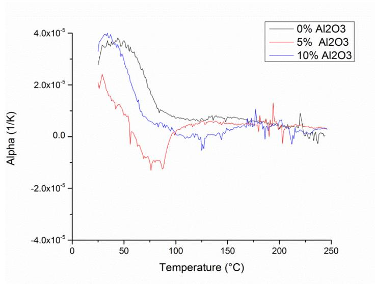
Fig. 37 *Overall CTE temperature variations after low temperature exposure*
