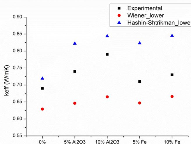
Fig. 38 *Effective thermal conductivities – experimental vs. theoretical predicted*
