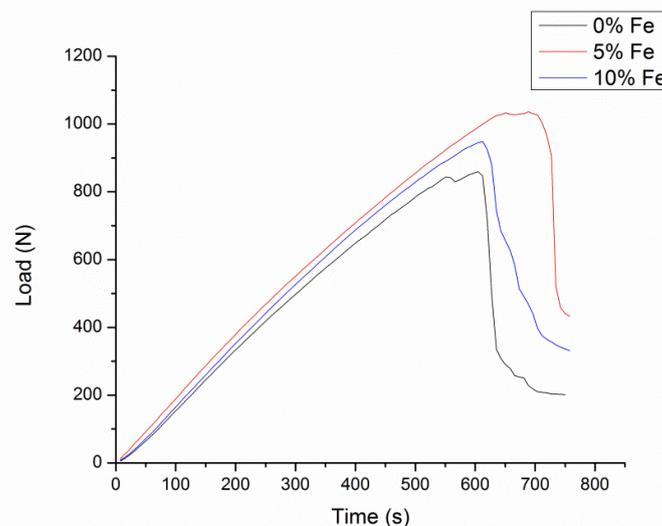
Fig. 12 *Load vs. time evolution curves on low temperature preconditioned iron particles reinforced hybrid polymer specimens in flexure*
