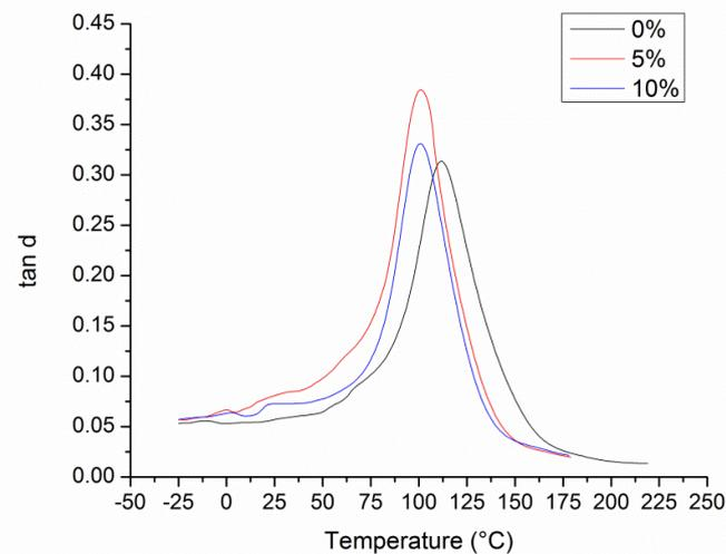
Fig. 18 Damping factor variation with temperature in particle-fiber hybrid architectures
