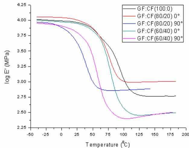
Fig. 23 Reinforcements' volume fraction and UD fiber orientation effects on the storage modulus at different temperatures
