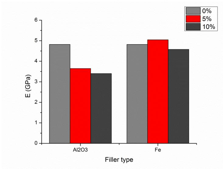
Fig. 4 Particle-fiber hybrid composites' Young modulus from tensile tests
