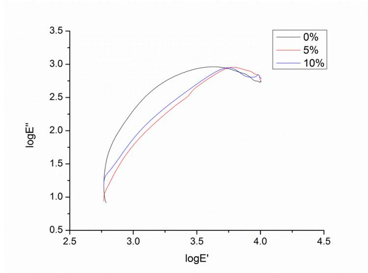
Fig. 19 Cole-Cole diagrams for the particle-fiber polymer composites
