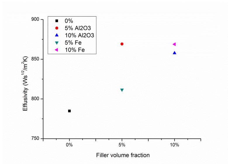
Fig. 40 Thermal effusivity experimental values of the hybrid composite structures
