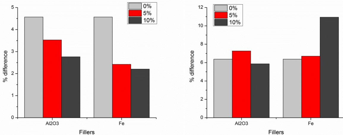
Fig. 13 *Percent difference between Young modulus in flexure: room and low temperature conditioned (left); room and temperature range (right)*
