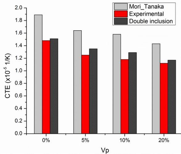
Fig. 50 CTE mean experimental values vs. micromechanical predicted
