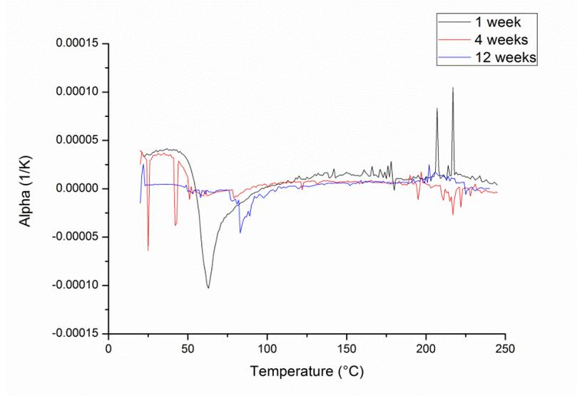
Fig. 30 CTE temperature variations in reference specimens subjected to water exposure
