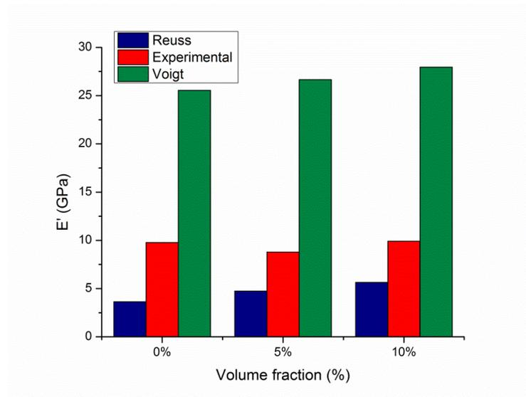
Fig. 20 Theoretical vs. experimental data values accounting for different particle fractions
