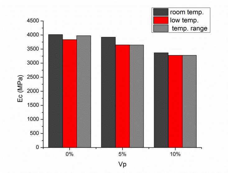
Fig. 11 *Mean elastic modulus in flexure for  $\text{Al}_2\text{O}_3$  fillers hybrid composites*
