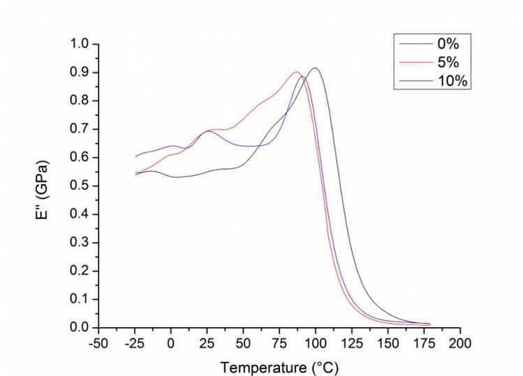
Fig. 17 Particle content effects on the loss modulus at different temperatures
