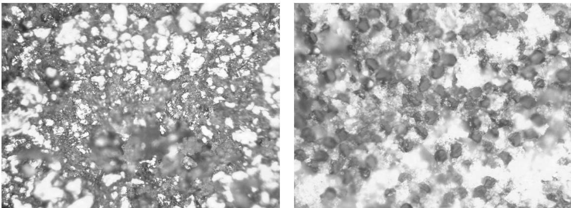
Fig. 1 *Micrographic views on particle-particle (left) and particle-fiber (right) hybrid composites developed*
