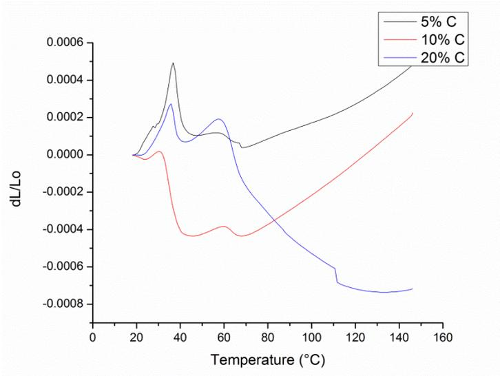
Fig. 48 Thermal strain fields developed within hybrid composites during heating
