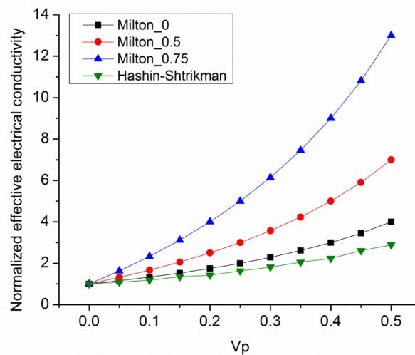
Fig. 55 *Effective electrical conductivity function of relative iron particle content in hybrid iron-graphite reinforced PVAc based composites*
