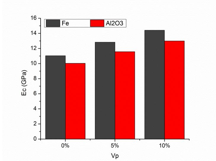
Fig. 9 *Theoretical predicted values based on the multi-step homogenization scheme used for particle-fiber reinforced polymer composites*
