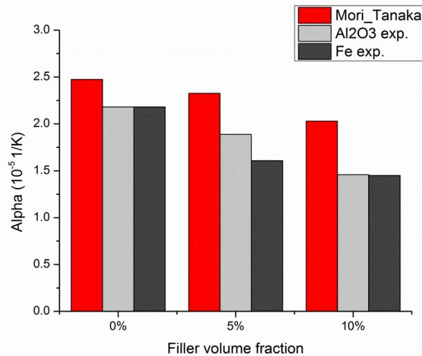
Fig. 28 Comparison on theoretical predicted vs. experimental retrieved CTE values
