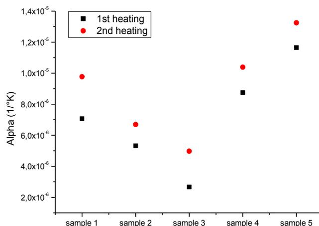
Fig. 27 Instantaneous CTE values (at 25 °C) for samples undergoing two successive scans
