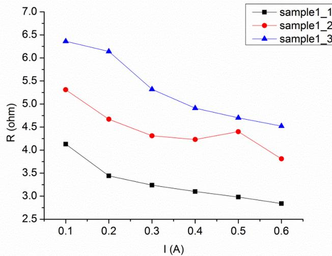
Fig. 51  $R(I)$  variation with applied current intensity for multi-phase composite specimens
