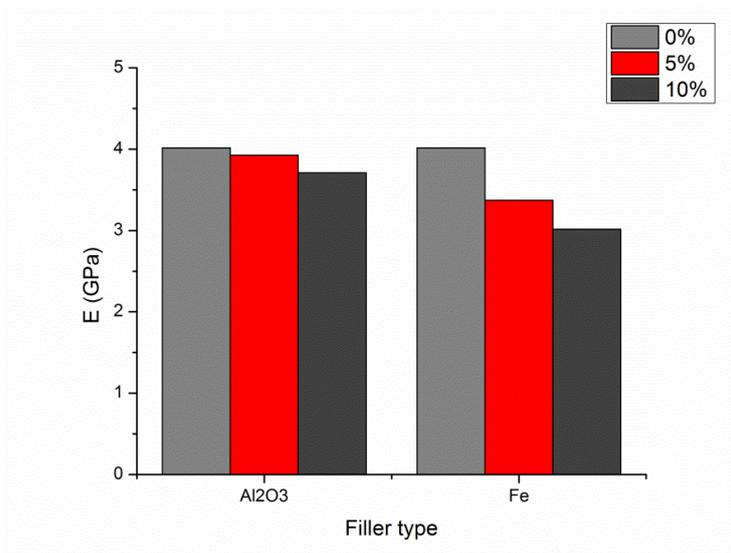
Fig. 6 Particle-fiber hybrid composites' Young modulus in flexure
