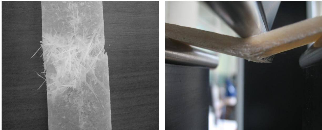
Fig. 2 Composite breakage in tensile (excerpt, left) and flexure (right)
