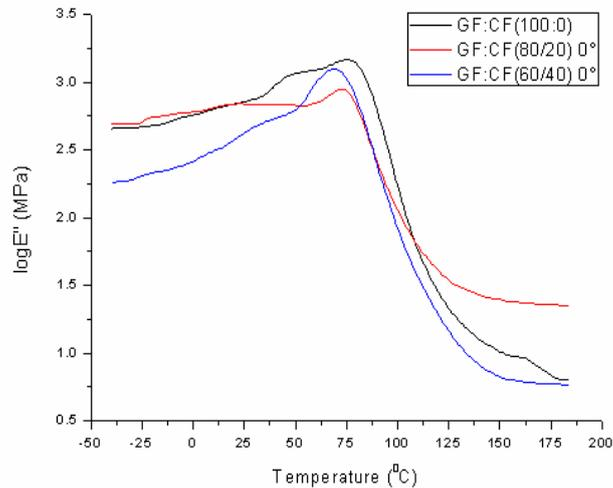
Fig. 24 Reinforcements' volume fraction and UD fiber orientation effects on the loss modulus at different temperatures
