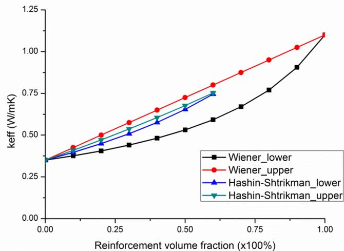
Fig. 41 Lower and upper thermal conductivity bounds for E-glass fiber reinforced sample
