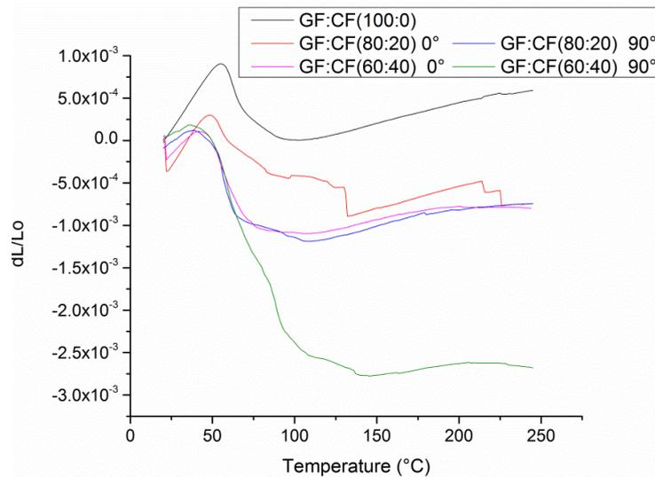
Fig. 42 *Thermal strain fields' evolution within the composite specimens*
