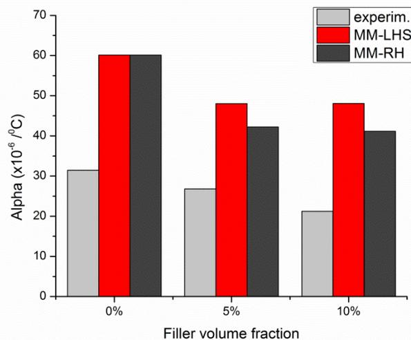
Fig. 35 *Theoretical predicted vs. experimental retrieved CTE values for  $\text{Al}_2\text{O}_3$  fillers*
