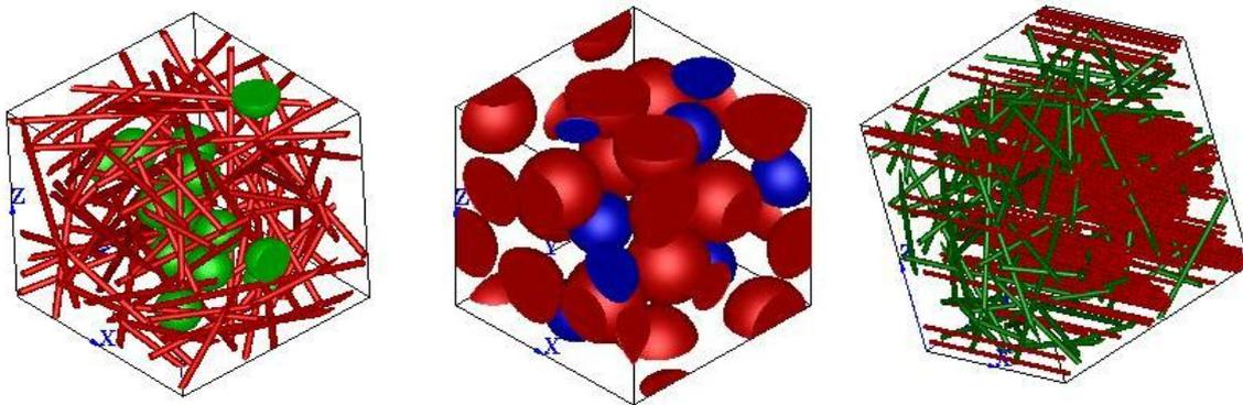
Fig. 3 RVEs used in effective material properties predictions in case of hybrid particle-fiber (left), particle-particle (middle) and fiber-fiber (right) architectures
