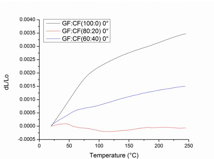
Fig. 44 *Thermal strain fields' evolution within the composite specimens*
