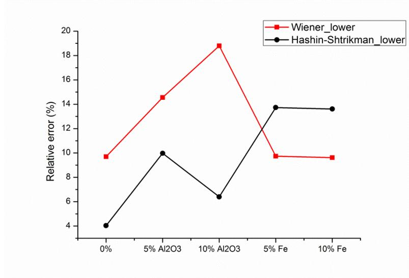
Fig. 39 Relative errors between the experimental and predicted thermal conductivities
