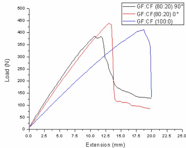
Fig. 14 Load vs. extension curves for unsymmetrical hybrid and reference composites in flexure
