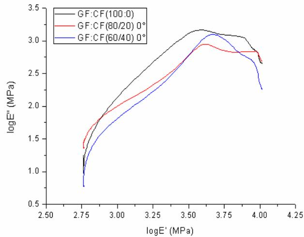
Fig. 26 (a) Cole-Cole diagrams in  $0^\circ$  oriented UD carbon fibers of hybrid fiber-fiber polymer composites
