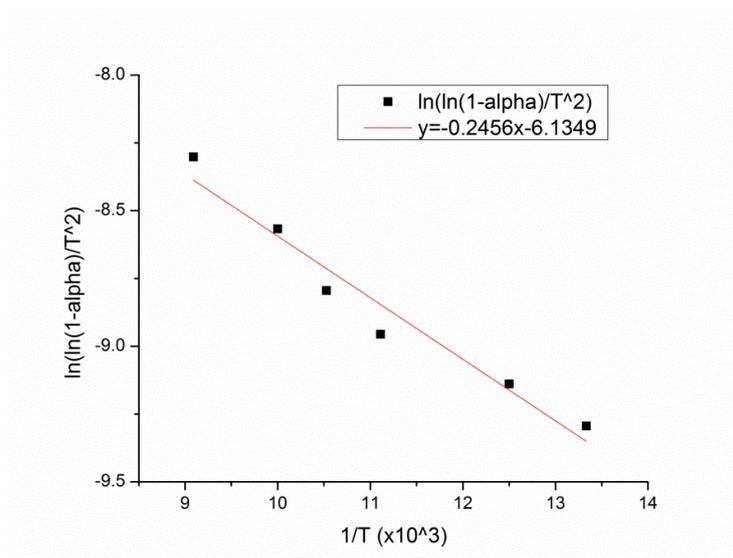
Fig. 22 Linear regression plots for activation energy identification
