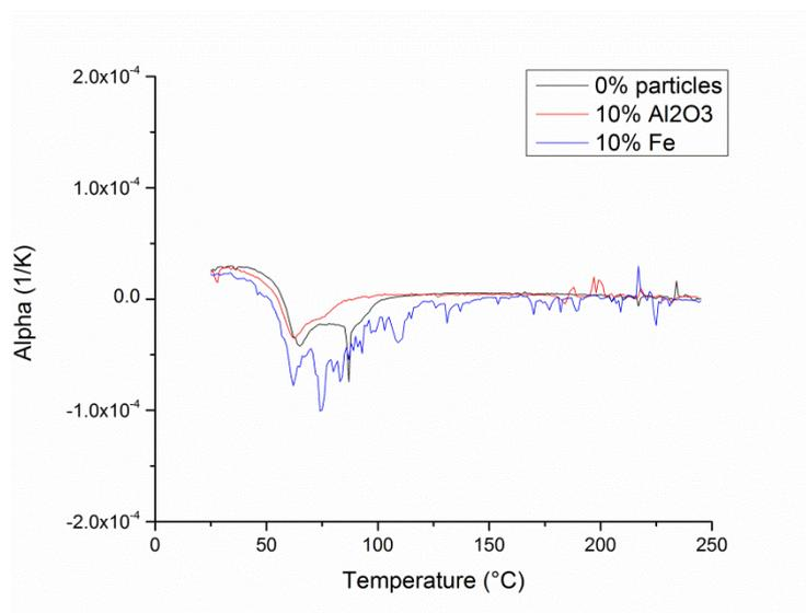
Fig. 34 *CTE temperature variations in samples prior subjected to temperature range*
