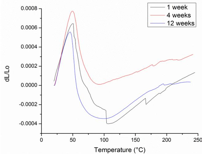
Fig. 32 Thermal strain fields' evolution within 10%  $Al_2O_3$  specimens under water exposure
