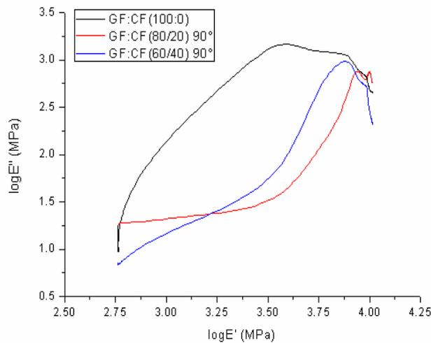
Fig. 26 (b) Cole-Cole diagrams in  $90^\circ$  oriented UD carbon fibers of hybrid fiber-fiber polymer composites
