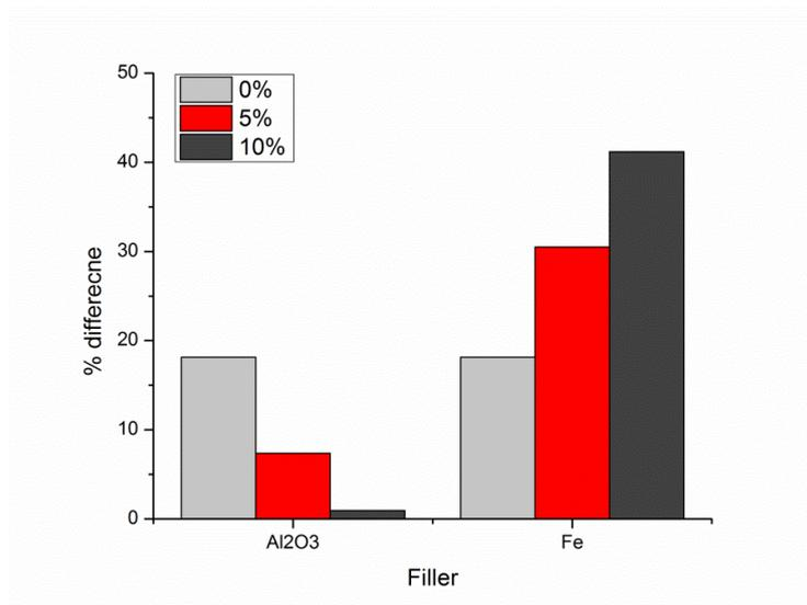
Fig. 8 *Percent difference between the experimental retrieved Young modulus from tensile and flexure testing*
