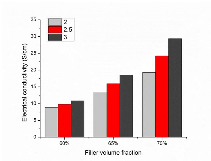
Fig. 57 *Effective predicted electrical conductivity values for different exponential values*
