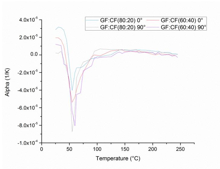
Fig. 43 *Instantaneous effective CTE temperature variations accounting different content and orientations of UD carbon fibres within the composite architectures*
