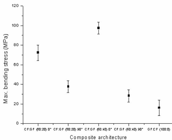
Fig. 15 Mean maximum bending stress values retrieved for the hybrid fiber-fiber polymer composite specimens
