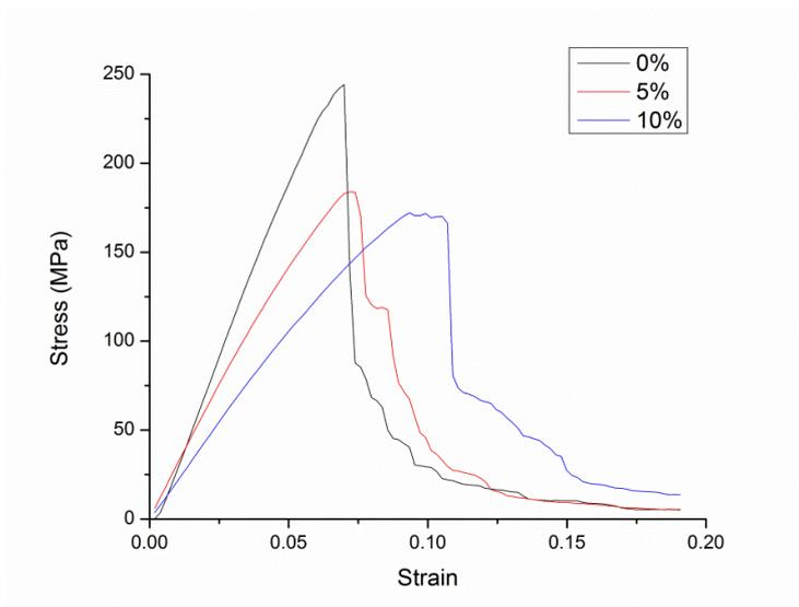
Fig. 7 Stress-strain curves from flexure tests on ceramic fillers hybrid composites
