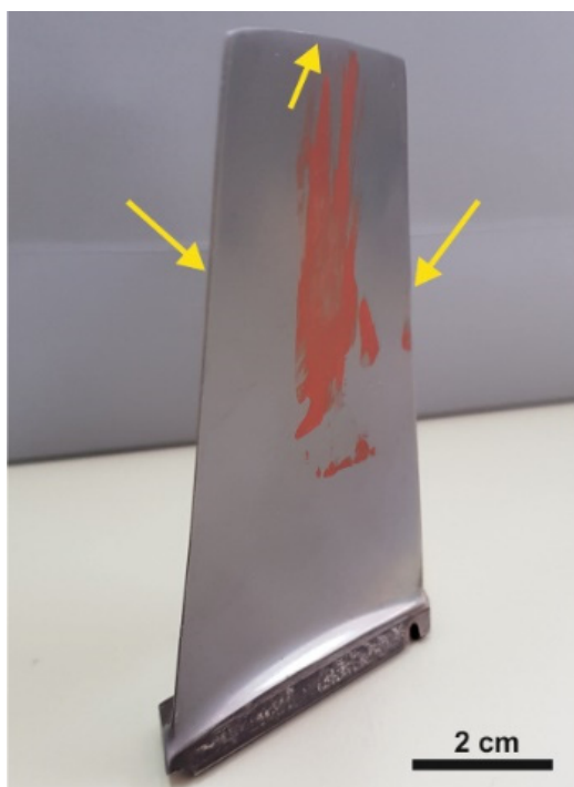
Fig. 4.9 Titanium jet engine blade (compressor blade); yellow arrows indicate the worn-out area [PRS19].
