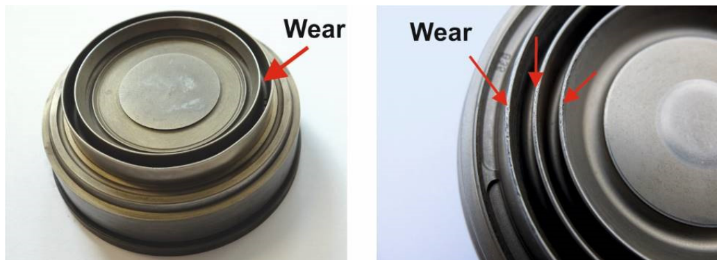
Fig. 4.1. Examples of compression mould with signs of wear [PSR19].
