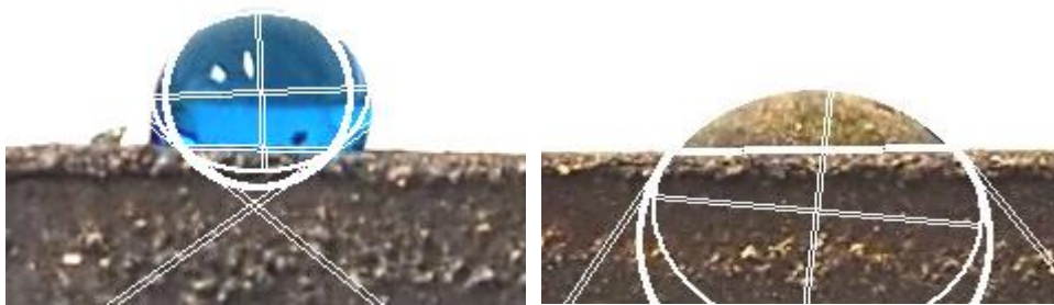
Figure 3.2.14 Representation of contact angles for P Cu7 (Roata, 2017b).
