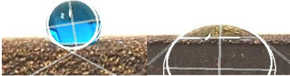
Figure 3.2.13 Representation of contact angles for P Cu2 (Roata, 2017b).
