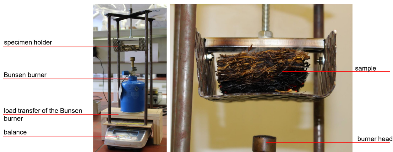
Figure 2.9: Own experimental setup and detailed view to determine the mass loss due to fire (Krenn et al. 2017a)
