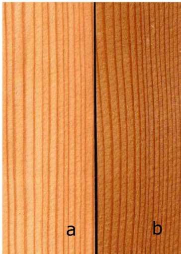
Larch heartwood samples before and after the light irradiation
