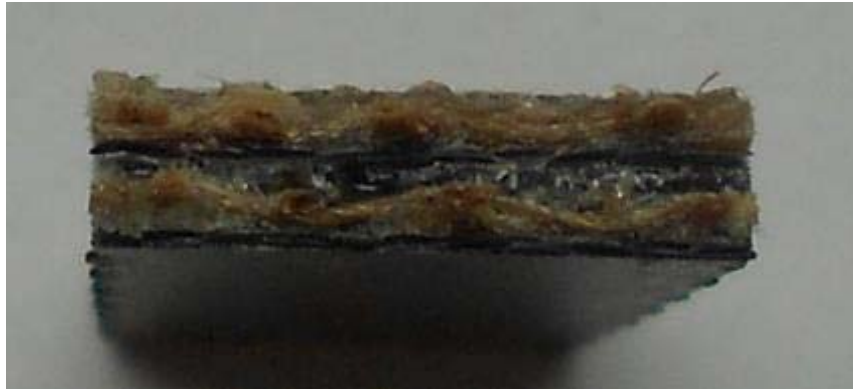
Figure 4.25 b. Cross-section through hybrid carbon-hemp composite panel
