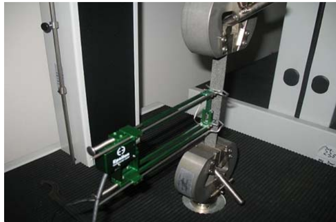
Figure 3.3. Tensile test detail on an epoxy impregnated 2/2 twill weave carbon fabric.
