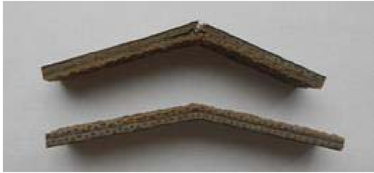
Figure 4.26 b. Carbon-hemp specimens after bending tests
