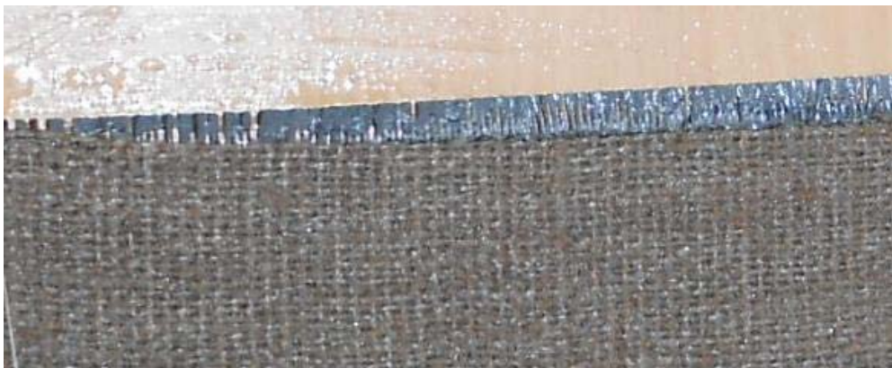
Figure 4.25 a. Hybrid carbon-hemp composite panel
