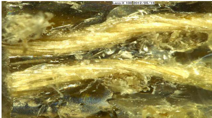
Figure 4.5. Cross-section through a hemp fabric based specimen irradiated with 56.7 kGy dosis (100X magnitude)
