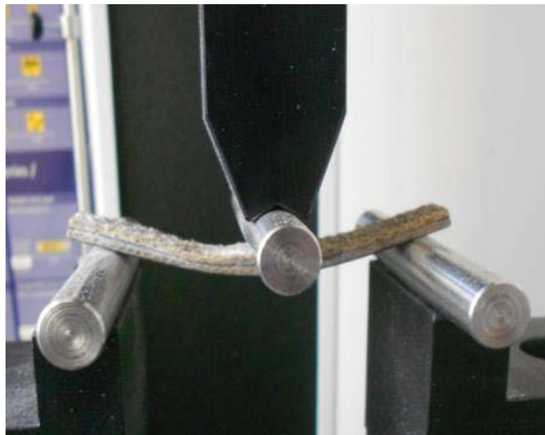
Figure 4.26 a. Carbon-hemp specimen during three-point bending test
