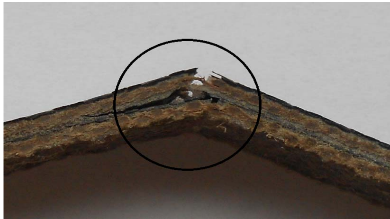
Figure 4.34. Side view of carbon-hemp fabric based specimens' break area
