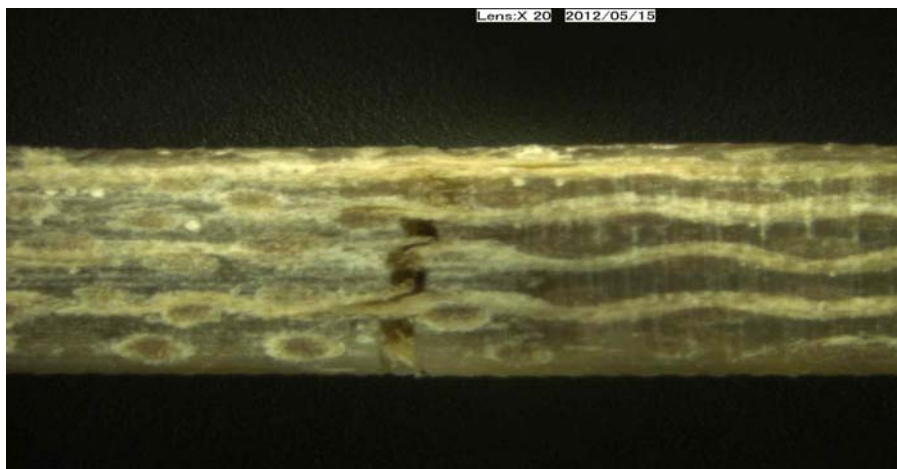
Figure 4.7. Side view of a non-irradiated hemp fabric based specimen (20X magnitude)
