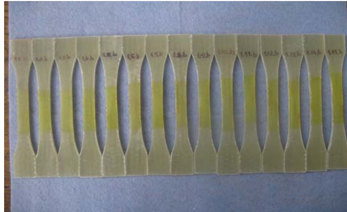
Figure 3.12. RT300 glass fabric-reinforced PolyLite 440-M888 polyester resin specimens cut on weft direction
