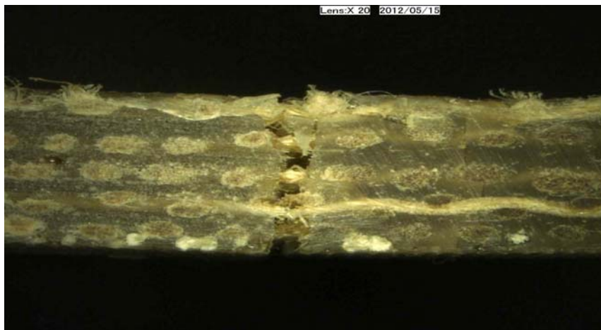
Figure 4.6. Side view of an irradiated hemp fabric based specimen (20X magnitude)
