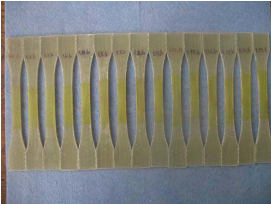
Fig. 6.3. RT300 glass fabric-reinforced PolyLite 440-M888 polyester resin specimens cut on weft direction
