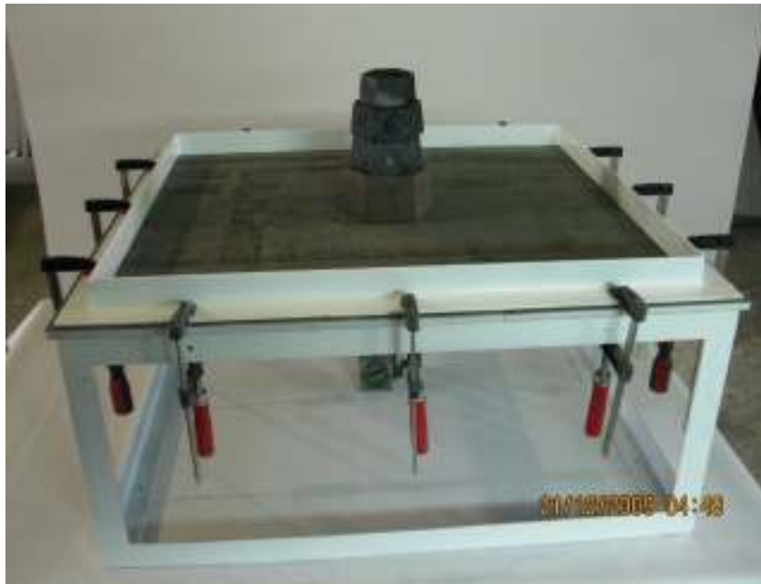
Fig. 7.2. Flexural load-unload test detail. Sandwich panel clamped on contour
