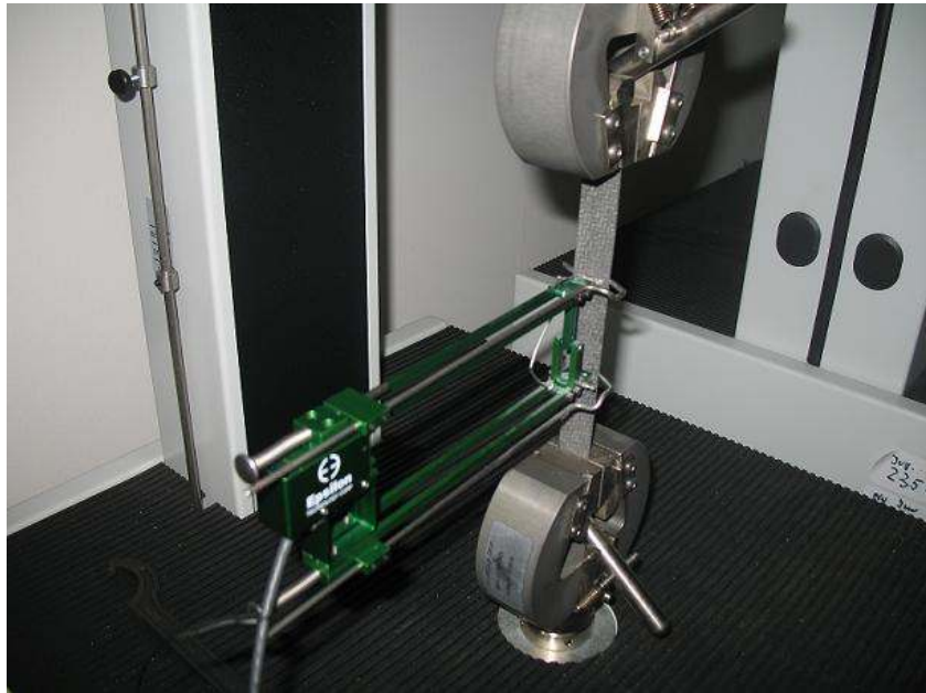
Fig. 7.4. Tensile test detail on an epoxy impregnated 2/2 twill weave carbon fabric
