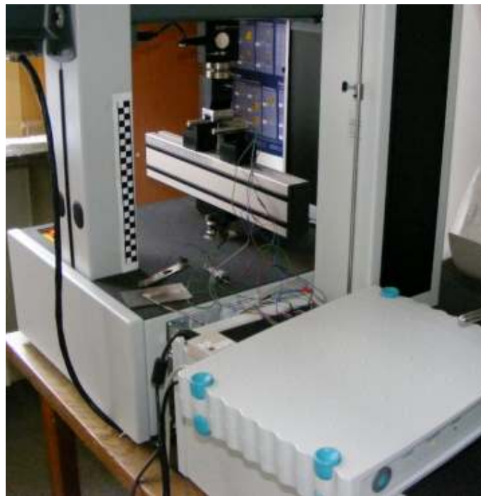
Fig. 6.1. Specimen connected to SPIDER8 device and subjected to four-point bend test
