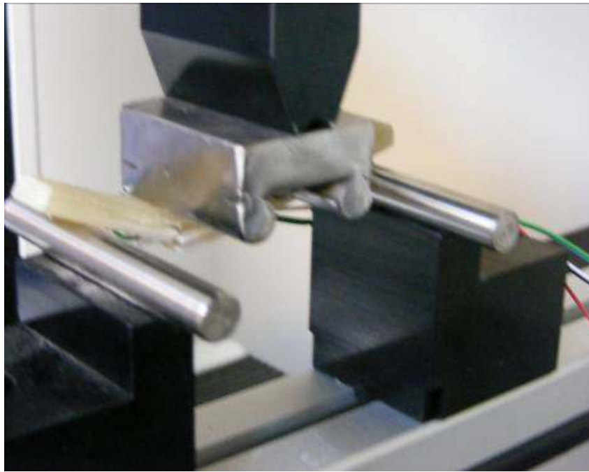
Fig. 6.2. Epoxy/CSM450 specimen with strain gages inserted between layers subjected to four-point bend test
