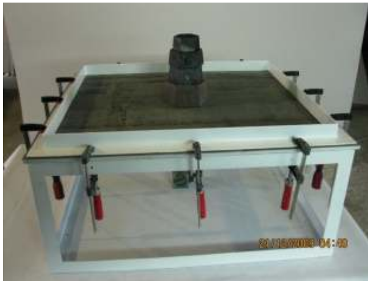
Flexural load-unload test detail. Sandwich panel clamped on contour
