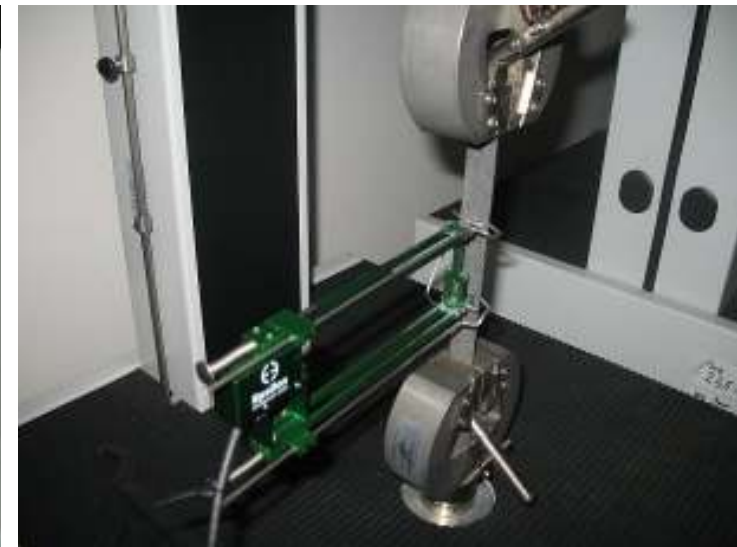
Tensile test detail on an epoxy impregnated 2/2 twill weave carbon fabric
