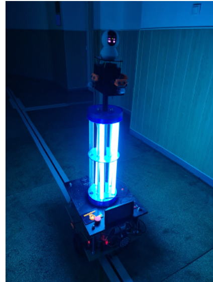
(b) RoboCoV Cleaner using markers to sterilize the hallway of Transilvania University of Brasov, 2021.
