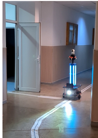
(d) RoboCoV Cleaner using markers placed on the floor and code QR placed on the door to make the decision at an intersection of the markers.
