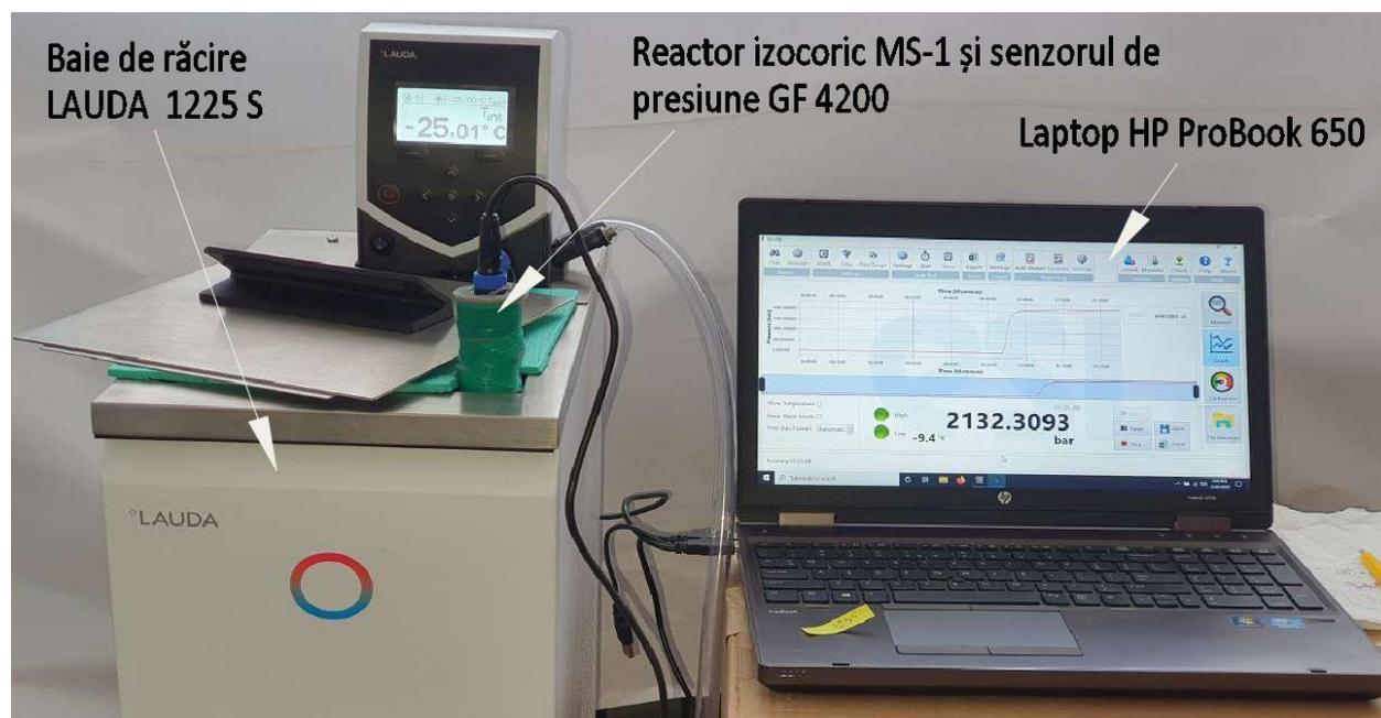
Figura 19- Equipment used to carry out experiments
