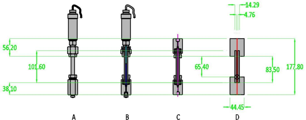
Figura 5– A) model reactor MS-1. B) reactor section MS-1 C) simplified reactor variant MS 1 D) model introduced in the simulation program
