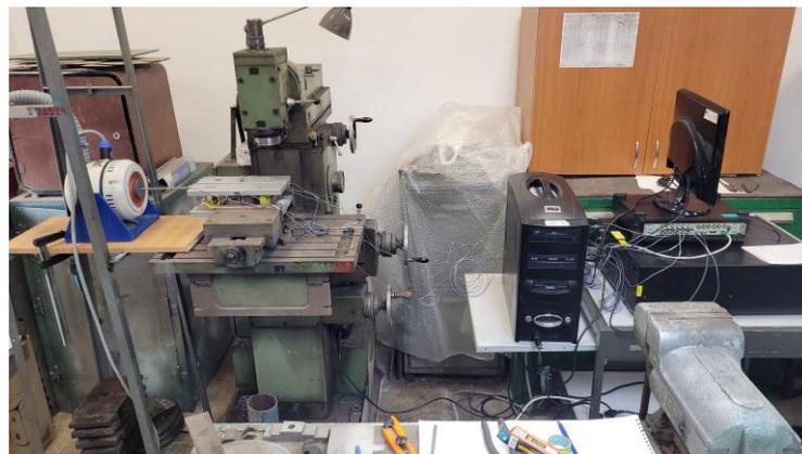
Figure 5.38 Modal test of dynamometer using shaker input signal in longitudinal direction (Ox – direction)
