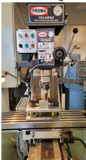
Figure 5.72 The dynamometer mounted on the table of milling machine-tool type PROMA FHV-50PD/2
