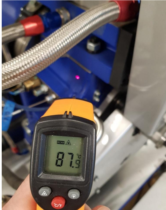
Fig. 2.23 Reading the exterior temperature of the AVL 5402 engine block
