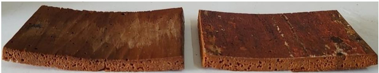
Fig.25. Significant warping after removal of the cut specimens from the water
