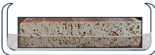
Fig. 19. Example of the immersion procedure of the samples.
