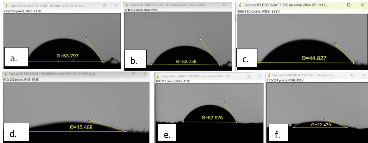
Fig. 40. a., b., c., d., f. Measurement of the contact angle for the three types of specimens: a., b. - healthy linden; c., d. - degraded linden; e., f. - Paulownia
