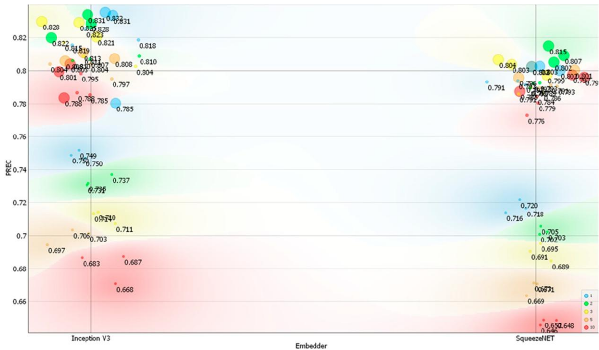
Figure 4.4. Precision (PREC) on the Posture dataset depending on the embedder used, the number of layers, and the number of neurons per layer. Legend: size of the data points represents the number of neurons used (small—10 neurons, medium—100 neurons, and large—1000 neurons) and color represents the number of layers used (red—ten, orange—five, yellow—three, green—two, and blue—one).
