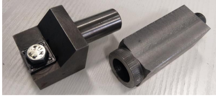
Fig. 7.6. The two bodies of the tool with a tangentially inclined edge
