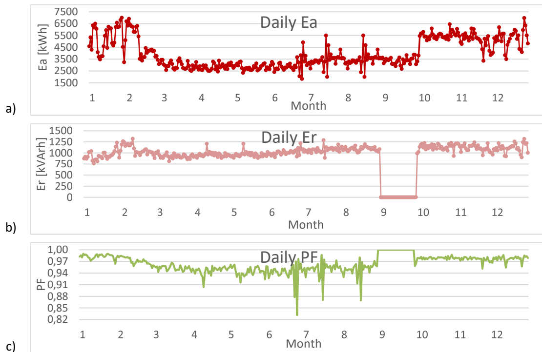
Fig. 4.19. Graph of data monitored with SCADA at the Măgurele Pumping Station in 2024 for: a) Active electrical energy, b) Reactive electrical energy, c) Power factor
