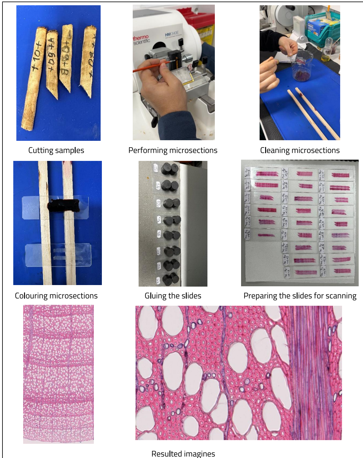
Figure 3.2. The working methodology applied in the anatomical analysis of wood (foto: Beşliu E.V.).
