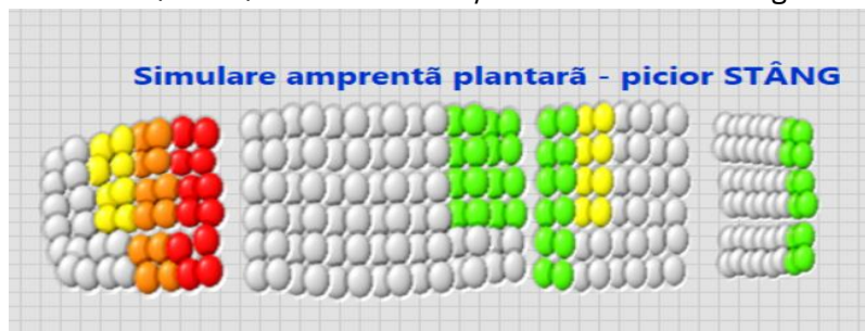
Fig. 3 Simulation of the plantar footprint of the left leg divided into the 4 zones with all 5 types of virtual LED entities
