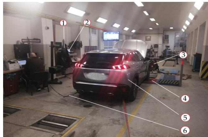
Fig. 4.2 - Experimental Research Laboratory: (a) Schematic Diagram of the Experimental Test Setup; (b) View of the Experimental Test Setup; 1. Connection Interface to the Vehicle's Electronic System (OBD II); 2. Control System; 3. Cooling Fans (2 Units); 4. Dynamometer Rollers Equipped with Eddy-Current Braking Systems; 5. Vehicle Under Test; 6. Exhaust Gas Sampling System for the Gas Analyzer.
