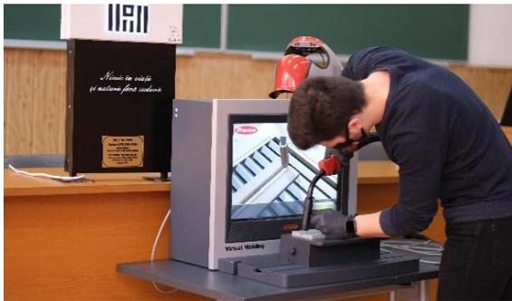
The *Virtual Welding* simulator is a system designed to train and improve the practical skills needed by the students in the specialization of Welding Engineering.
